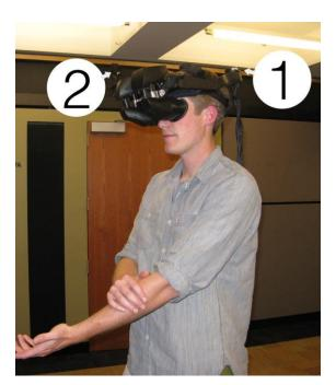
Figure 1. IVE equipment: (1) Head-mounted display, (2) Infrared cameras that track participant head movement
