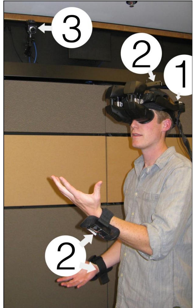
Figure 2. A participant during the experiment wearing the HMD (1), infrared tracking sensors on the head and hands (2), and cameras (3) that detect the position of the trackers.
