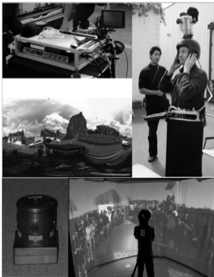
Figure 1 Top: recording in the field, left bottom: a stationary ODV “ladybug” camera, right bottom: ODV projected in a CAVE set-up
