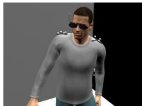
Figure 3 Representation of the subject's equipment, with markers attached to stereo glasses and a set of markers on each shoulder
