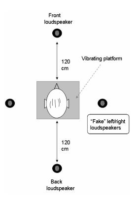
Figure 1 Top-view of the experimental setup
