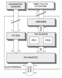
Figure 7: Data-glove electronics architecture.
