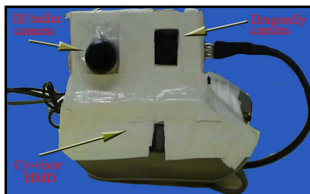
Figure 1. Capture and visualization system (Dragonfly camera, Infrared camera and the HMD)
