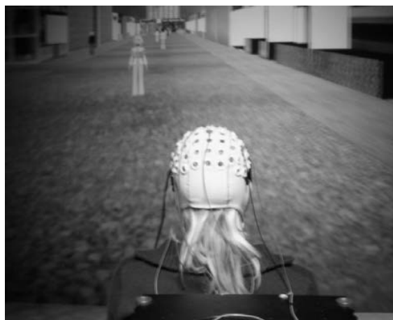
Figure 2: Participant in the virtual main street with shops and animated avatars during the Cave-FB. The subject wears an electrode cap (connected to the amplifier) and shutter glasses.
