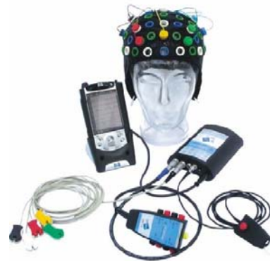
Fig. 2. Components of a Pocket PC based BCI system.
