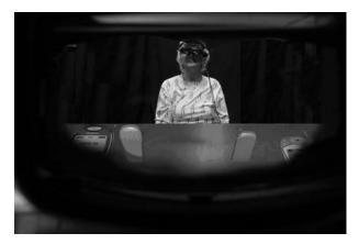
Figure 1. A photograph taken from the see-through HMD in the AR condition. The cellular phones on the table were virtual objects but the confederate and environment were directly visible and unmediated.
