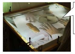
Projecting a synthesized video image of local and remote tabletop onto a screen over the table
