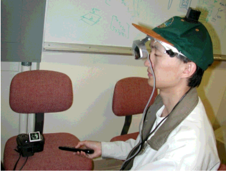
Figure 7: Immersive Remote Reality equipment. HMD, video camera, remote control and tracker (on top of HMD) are visible in photograph.
