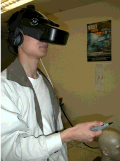
Figure 6: Virtual Environment equipment. HMD, stylus and tracker (on top of HMD) are visible in photograph.
