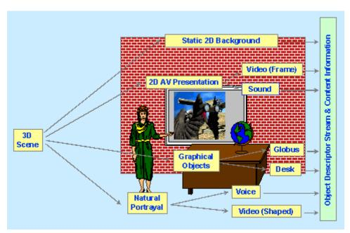
Fig. 1: Example of a BIFS scene graph in MPEG-4
