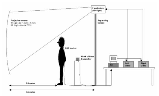
**Figure 1.** Schematic diagram of the laboratory set-up illustrating the observer's position in relation to the display. The observer's area of the laboratory was completely blacked out during the experimental sessions, with the only illumination coming from the projection display.
